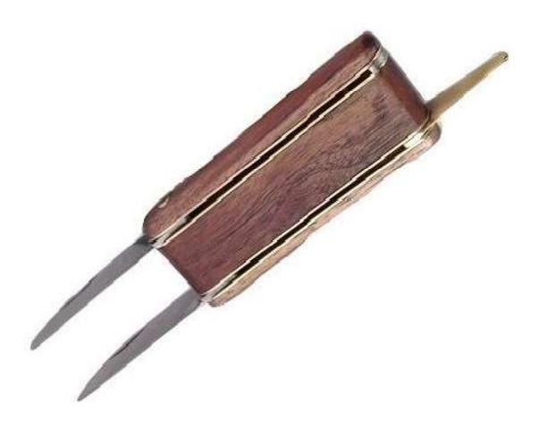
For the patch, flute and ring budding operation especially for removing the bud patches of same size from stock and scion
